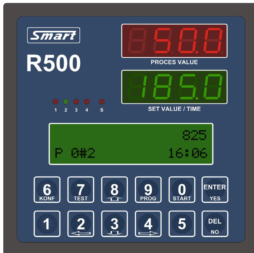
Fig. 1. R500 Programmable Regulator Front Panel
